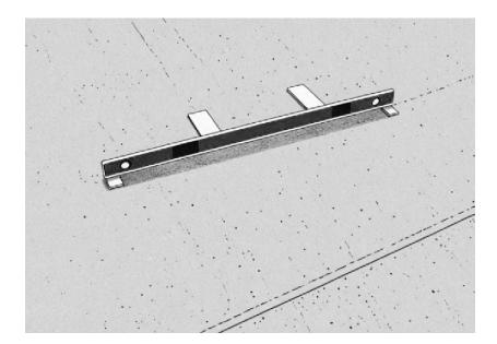
10. Now you are ready to install your mixture of mortar in the front and back edge of your columbarium. Use your template lined chocked on your cement pad for your mortar positioning
